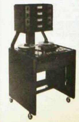
Electro Sound's 3.75/7.5 ips mastering recorder/reproducer, with frequency response to 18KHz at 3.75 ips, comes in several configurations for any needs.
